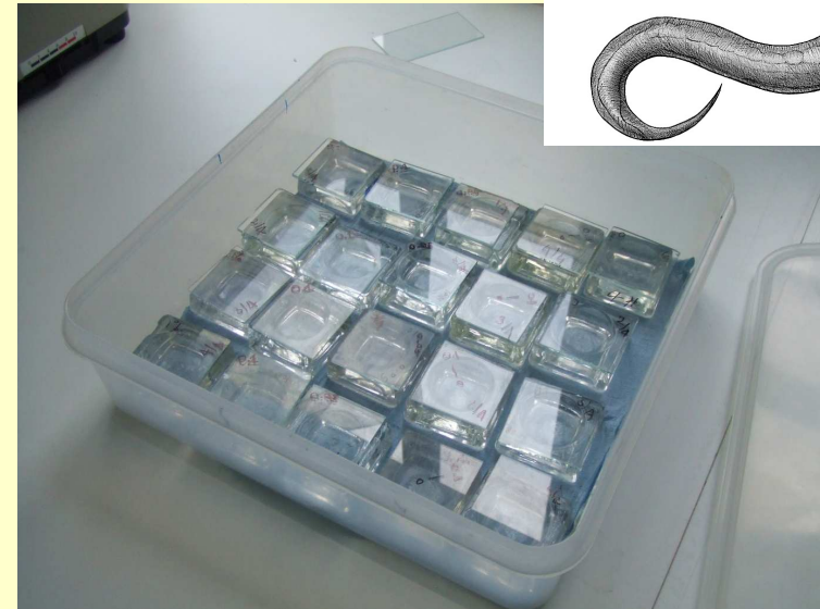
The soil nematode C. elegans is <1mm in length. Experiment undertaken in staining blocks in a humid chamber with 10 worms per block.
